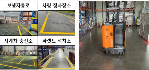
* Painting safety lines/marks * Installation of forklift LED beams
